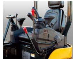
A tiltable left-side console allows the operator easier access to the cab. A safety lock system is designed to prevent exiting the cab while hydraulic controls are live. When the safety lever and left side console are positioned upright, hydraulic functions are disengaged.
